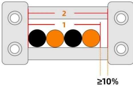
$$(\text{拖链内宽}4) \geq (\text{线缆并列后宽度}5) \times 10\%$$
