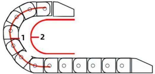
$$(\text{拖链弯曲半径}1) \geq (\text{线缆弯曲半径}2) \times 10\%$$
