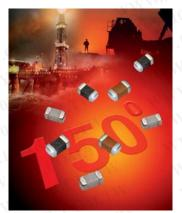
AVX has developed a range of multilayer ceramic capacitors designed for use in applications up to 150°C. These capacitors are manufactured with an X8R and an X8L dielectric material. X8R material has capacitance variation of  $\pm 15\%$  between -55°C and +150°C. The X8L material has capacitance variation of  $\pm 15\%$  between -55°C to 125°C and +15/-40% from +125°C to +150°C.
