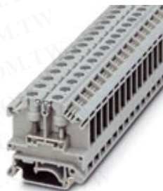
Universal terminal block with bolt connection, cross section: 0.1 - 2.5 mm 2 , width: 9 mm, color: Gray
