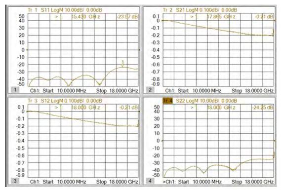
Note: S11/S12/S21/S22 plots shown represent IL and VSWR of two adaptors tested. To extract IL of a single adaptor divide IL measured by two.
