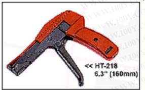
FOR CABLE TIE FROM 2.2 TO 4.8mm.WIDTH, AND THICKNESS UP TO 1.6mmFASTEN AND AUTOMATIC CUT HT-218 TIES, WITHADJUSTABLE BUNDLING PRESSURE.
