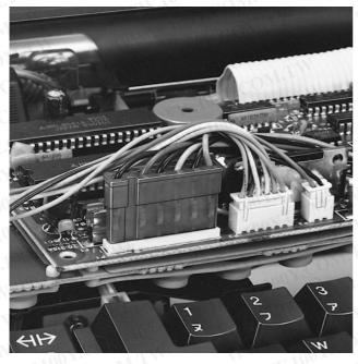
The V connector can have from two to six circuits. A single contact position is provided 7.5mm away from the adjacent position, while the pitch of other positions is 5.0mm. This prevents reverse connection of the receptacle and header.
