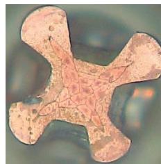
Uneven Crimp and Wall Thickness
