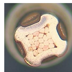
Crimp Too Loose and Void on Within Crimp
