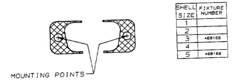
VIBRATION LEVEL IS APPLIED TO THE CONNECTOR MOUNTING AREA (XXXXX) OF THE VIBRATION FIXTURE.
