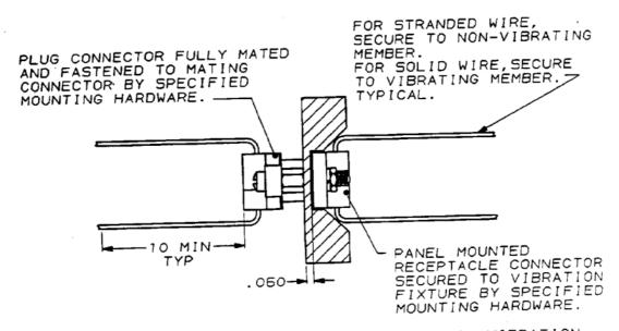
NOTE: RECEPTACLE CONNECTOR TO BE MOUNTED ON VIBRATION FIXTURE UNLESS OTHERWISE SPECIFIED.
