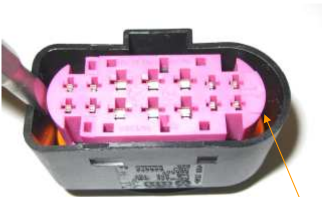
Figure 4: 14 posn, receptacle housing, radial seal, Junior-Power-Timer, Micro-Timer II Contact insertion
