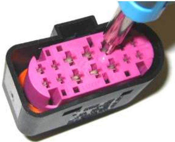
Figure 7: 14 posn, receptacle housing, radial seal, Junior-Power-Timer, Micro-Timer II Contact extraction
