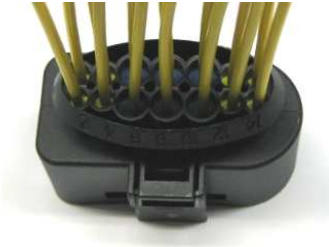
Figure 3: 14 posn, receptacle housing, radial seal, Junior-Power-Timer, Micro-Timer II Contact insertion
