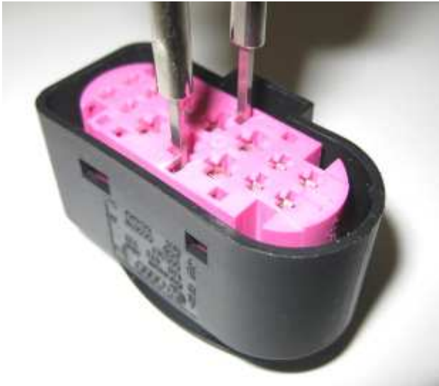
Figure 5: 14 posn, receptacle housing, radial seal, Junior-Power-Timer, Micro-Timer II Contact extraction
