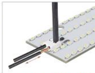
Inserting/removing fine-stranded conductors by lightly pressing on push-button (e.g. using a 206-860 operating tool).
