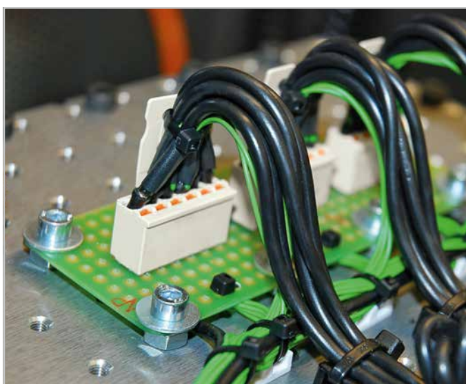
Vibration test performed on a picoMAX® eCOM wire-to-board connection (2091 Series)
