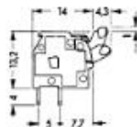
Diameter of drilled holes: 1.1 +0.1 mm
