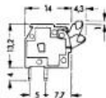
Diameter of drilled holes: 1.1 +0.1 mm
