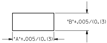
RECOMMENDED PANEL OPENING (SCALE 2:1)
