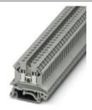
Feed-through terminal block, nom. voltage: 690 V, nominal current: 24 A, connection method: Screw connection, number of connections: 2, cross section:0.2 mm<sup>2</sup> - 4 mm<sup>2</sup>, AWG: 24 - 12, width: 6.2 mm, color: gray, mounting type: NS 35/7,5, NS 35/15
