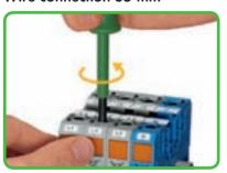
Counter-clockwise rotation using a screwdriver (blade width 5.5 mm). Hold clamp in open position using the latch.
