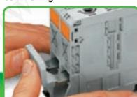
Commoning with adjacent umper. Insertion of jumper above the conductor entry hole, without tools. Rated cross section is still  $50 \text{ mm}^2/AWG 2/0 \text{ and}$ 95 mm<sup>2</sup>/AWG 4/0.
