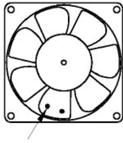
Note: The glues on the impeller is for impeller balance. Please don't remove it.
