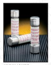
Tri-onic TRM time-delay midget fuses are rated 250 volts AC and are offered in ampere ratings from 1/10A to 30A. They have 12 seconds time delay at 200% rating to provide supplemental protection of small motors, small transformers and other high inrush loads, plus many other 250 volt applications. (Not for Branch Circuit Protection).
