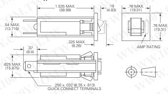
1. Soldering to terminals is not recommended. 2. Recommended Panel Thickness: Style Q: .032" - .062" (.813 mm - 1.574 mm) .075" - .105" (1.905 mm - 2.667 Style T:
