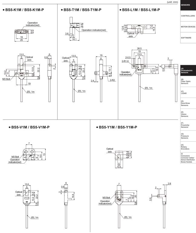
% When using photoelectric sensors closely over two units, it may result in malfunction due to mutual interference. When installing the product, tighten the screw with a tightening torque of 0.49N·m.
