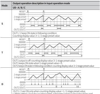
OUT1/2 are ON only when counting display value = 1/2-stage preset value. • When setting 1 kcps for counting speed, solid state contact output should be used. When using contact output, it is difficult to execute normal output operation due to contact reaction time.
