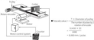
Select decimal point: -----, prescale decimal point: ----- and set prescale value: 0.069, it is available to control conveyor position by 0.1 mm unit. Select decimal point: -
