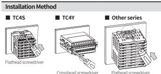
Mount the product to panel with bracket, push it to arrow direction by using screw driver. • In case of TC4Y Series, fasten the bolts.
