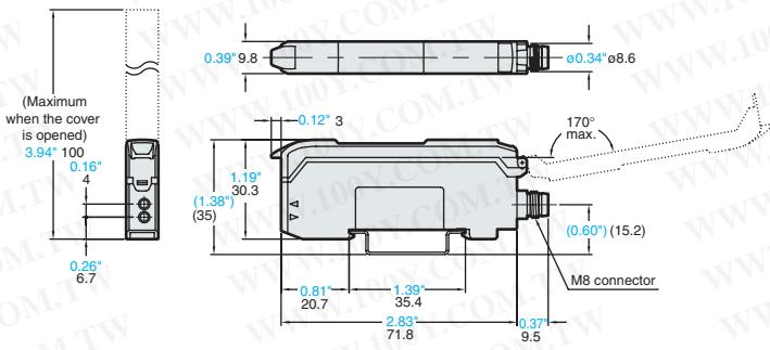
When the mounting bracket (Optional) OP-73880 is attached:
