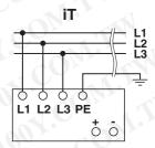
The connection for 3x 400 V AC ... 500 V AC is established using the L1, L2, L3 and PE screw connections. The device can be connected to a 3-phase system with nominal voltages of 3x 400 V AC ... 500 V AC. In the event of a phase failure, unrestricted operation is possible with nominal capacity.
