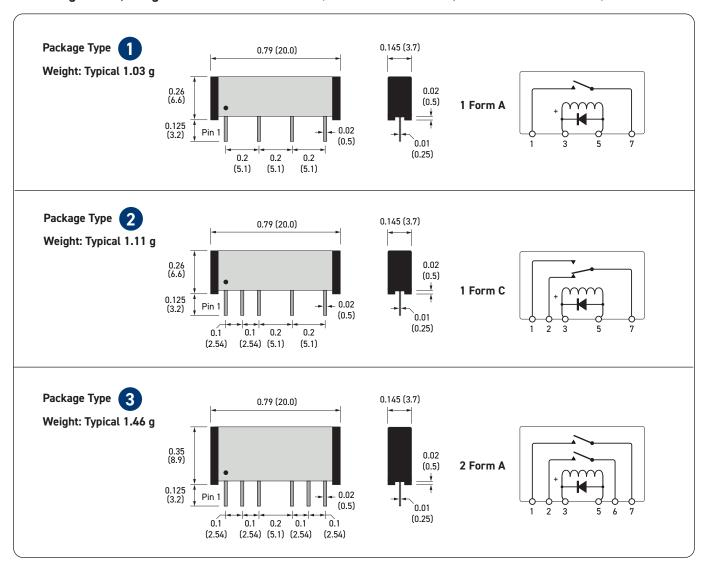
**Important:** Where the optional internal diode is fitted or for all Form B types, the correct coil polarity must be observed, as shown by the + symbol on the schematics.
