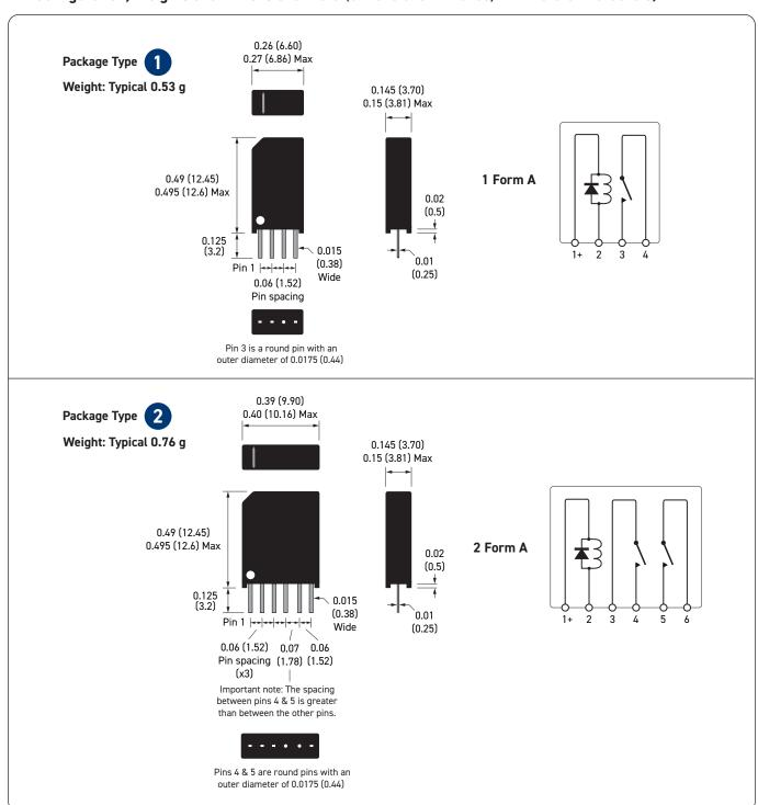
Pin Configuration, Weights and Dimensional Data (dimensions in inches, millimeters in brackets)
