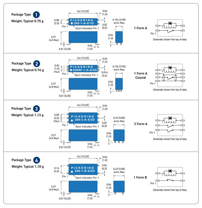
Important: When an optional internal diode is fitted the orientation spot end of the relay forms the positive connection.
