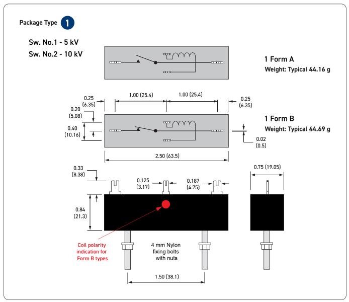
Series 62: Pin Configuration, Weights and Dimensional Data (dimensions in inches, millimeters in brackets)
