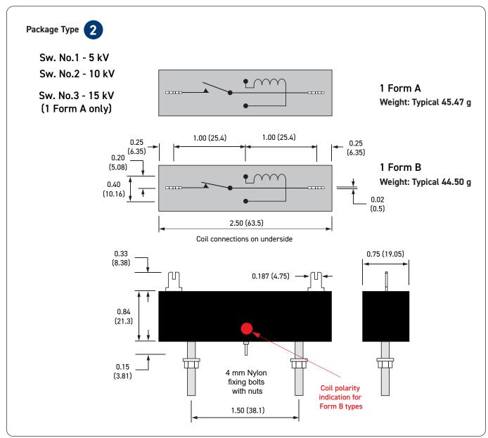
Series 63: Pin Configuration, Weights and Dimensional Data (dimensions in inches, millimeters in brackets)
