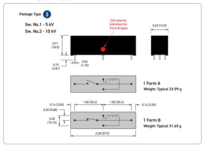
**Important:** For all Form B types, the correct coil polarity must be observed. The positive connection is shown by the red spot on the package.
