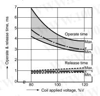
4.-(2) Operate & release time (without diode, 1 Form A 1 Form B) Tested sample: DSP1-DC12V, 5 pcs.
