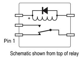
**Important:** When an optional internal diode is fitted the orientation spot end of the relay forms the positive connection.
