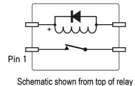
**Important:** When an optional internal diode is fitted the orientation spot end of the relay forms the positive connection.
