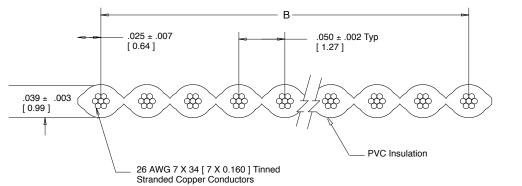
Note: Red marking on one edge of cable designates wire #1.
