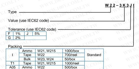
For CECC released product state on order the CECC number and style. Example: **W22-3K3JI CECC40201-002 JB** For SnPb finish instead of Pb-free replace the packing suffix with **PB**. Example: **W22-3K3JPB**
