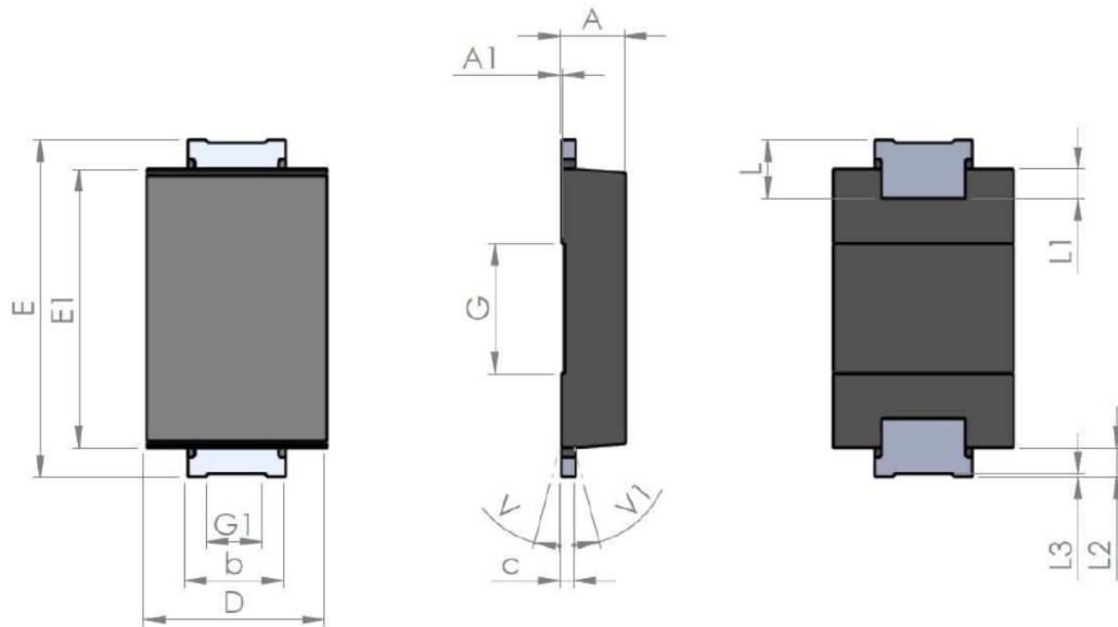
Table 5. SMA Flat Notch package mechanical data
