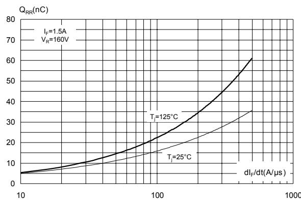
**Figure 10. Reverse recovery time versus dI\_F/dt (typical values)**
