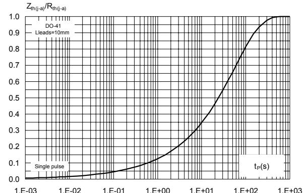
**Figure 7. Relative variation of thermal impedance junction to lead versus pulse duration (DO-15)**
