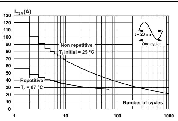
**Figure 7. Non repetitive surge peak on-state current and corresponding values of I<sup>2</sup>t**
