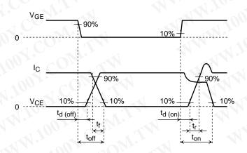
Note 2: Switching loss measurement waveforms
