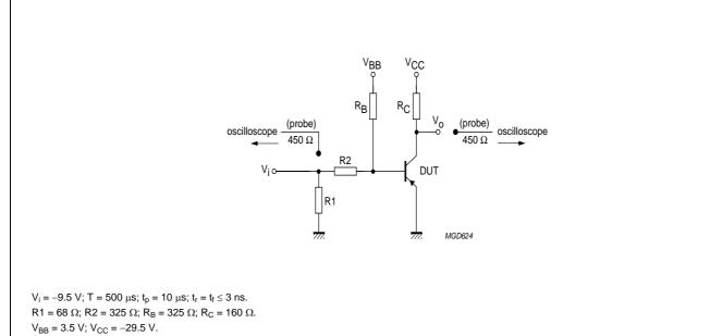
Fig.2 Test circuit for switching times.
