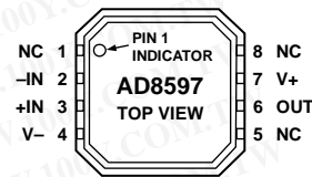
Figure 1. AD8597 8-Lead SOIC (R-8)
