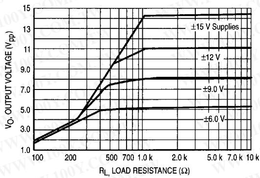
**Figure 9. Negative Output Voltage Swing
