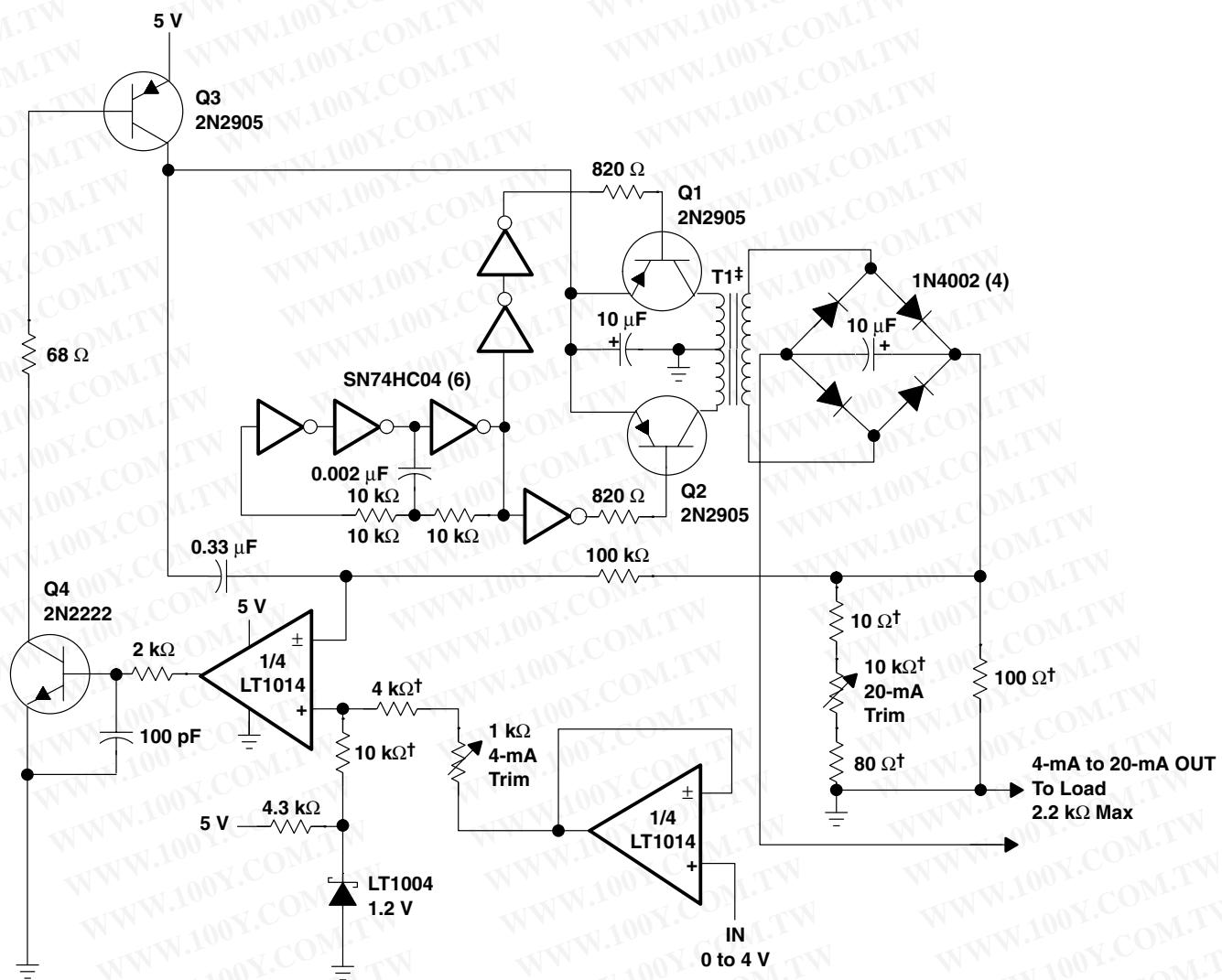
† 1% film resistor. Match 10-kΩ resistors 0.05%.
