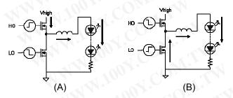
Fig.2 (A) Storing Energy in Inductor (B) Releasing Inductor Stored Energy
