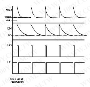
Fig.8 Open Circuit Fault Signals, with Clamp
