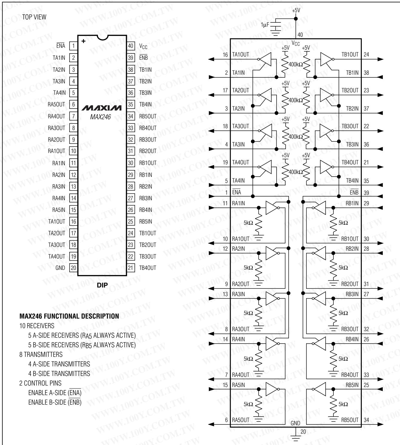
Figure 22. MAX246 Pin Configuration and Typical Operating Circuit
