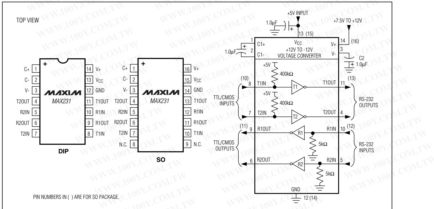
Figure 10. MAX231 Pin Configurations and Typical Operating Circuit
