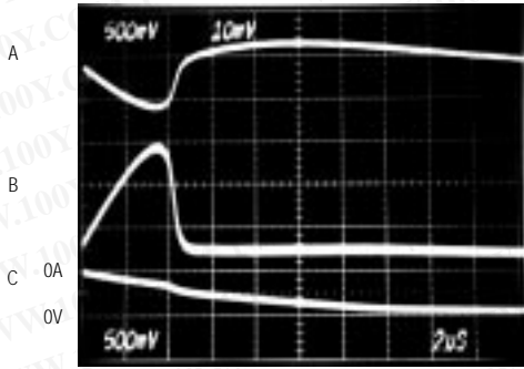
CURRENT-LIMIT RESPONSE (MAX891L, R_L = 0.8\Omega )
