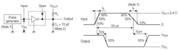
Note 1: Pulse Width 50  $\mu$ s, Duty Cycle 10%
