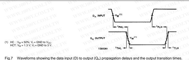
Fig. 7 Waveforms showing the data input (D) to output ( $Q_n$ ) propagation delays and the output transition times.
