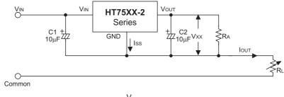
$$I_{OUT} = \frac{V_{XX}}{R_A} + I_{SS}$$
