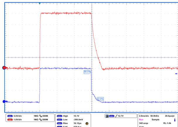
Figure 23. Turn-on time ( $V_{OUT} = 1.2 V$ )
