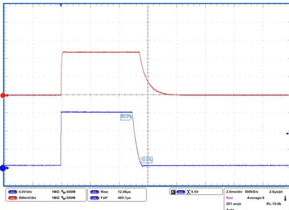
Figure 24. Line transient ( $V_{OUT} = 5 V$ )
