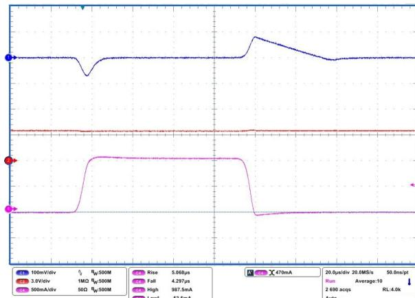
$V_{IN} = 3.5 V$ ,  $I_{OUT}$  = from 10 mA to 1.2 A,  $C_{IN} = 1 \mu F$   $C_{OUT} = 4.7 \mu F$ ,  $t_{rise} = 5 \mu s$
