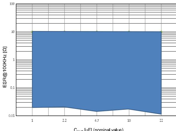
Figure 21. Stability plan ( $V_{OUT} = 1.2 V$ )
