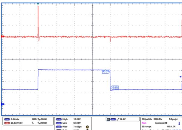
Figure 25. Line transient ( $V_{OUT} = 1.2 V$ )
