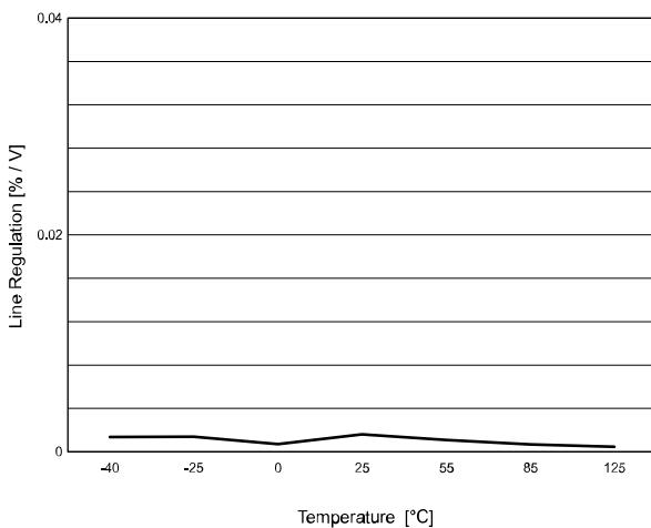
**Figure 9. Line regulation vs. temperature ( $V_{IN} = 2.5$  to  $18$  V,  $V_{OUT} = 1.2$  V,  $I_{OUT} = 10$  mA)**
