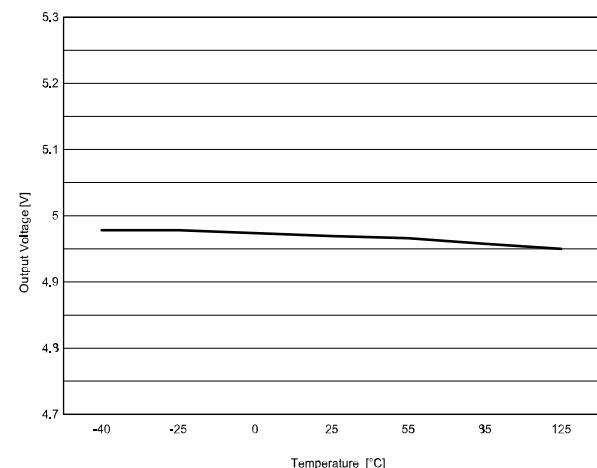
**Figure 8. Line regulation vs. temperature ( $V_{IN} = 6$  to  $18$  V,  $V_{OUT} = 5$  V,  $I_{OUT} = 10$  mA)**
