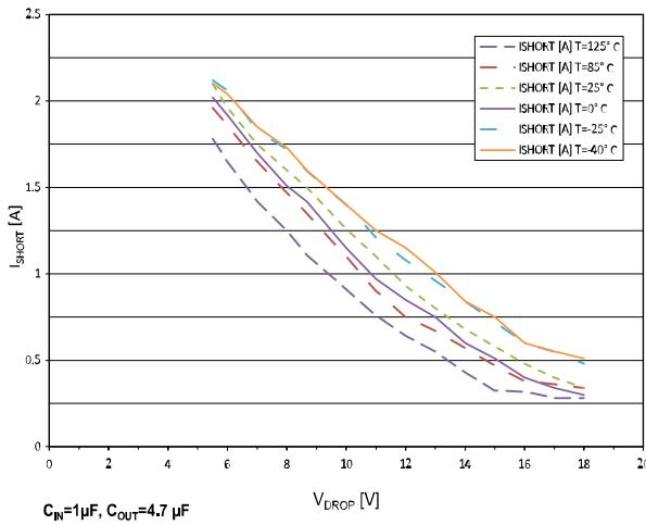
**Figure 17. Short-circuit current vs. dropout voltage ( $V_{OUT} = 1.2 V$ )**
