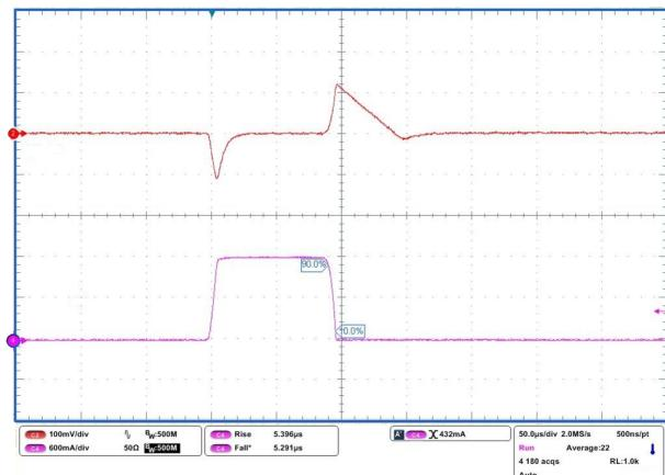
$V_{IN} = 6 V$ ,  $I_{OUT}$  = from 10 mA to 1.2 A, NO  $C_{IN}$ ,  $C_{OUT} = 4.7 \mu F$ ,  $t_{rise} = 5 \mu s$
