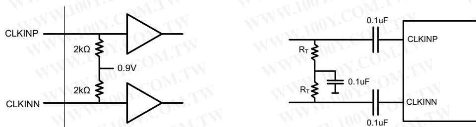
Figure 35. Recommended Differential Clock Driving Circuit
