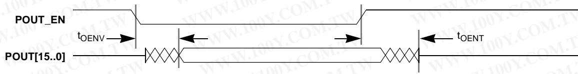
Figure 11. CLC5903 Parallel Output Enable Timing
