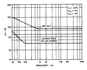
Figure 4. Noise Spectral Density vs. Frequency
