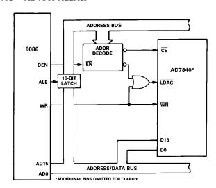
Figure 18. AD7840-8086 Parallel Interface
