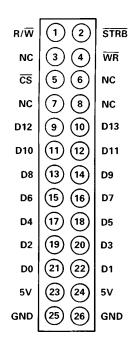
Figure 29. SKT4, IDC Connector Pinout
