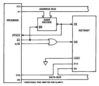
Figure 19. AD7840-MC68000 Parallel Interface
