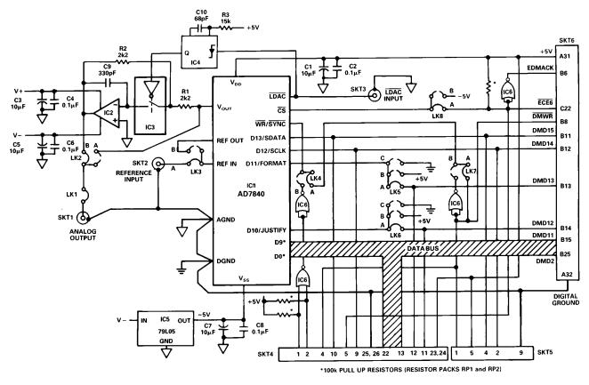
Figure 25. Data Acquisition Circuit Using the AD7840
