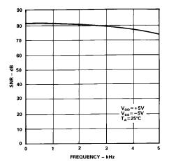
Figure 13. Performance vs. Frequency (No Sample-and-Hold)
