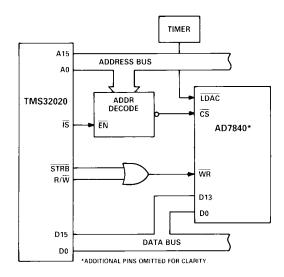
Figure 17. AD7840-TMS32020 Parallel Interface
