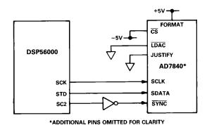
Figure 21. AD7840-DSP56000 Serial Interface
