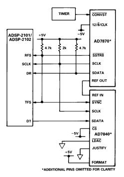
Figure 20. Complete DAC/ADC Serial Interface
