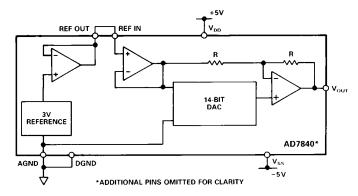
Figure 5. AD7840 Basic Connection Diagram
