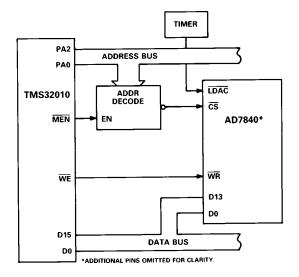
Figure 16. AD7840-TMS32010 Parallel Interface
