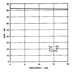
Figure 14. Performance vs. Frequency (with Sample-and-Hold)
