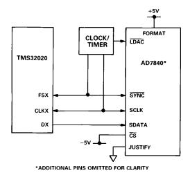
Figure 22. AD7840-TMS32020 Serial Interface
