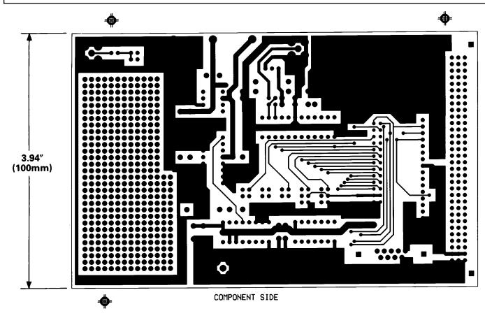
Figure 27. PCB Component Side Layout for Figure 25
