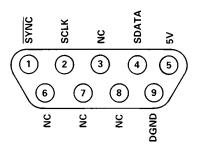
Figure 30. SKT5, D-Type Connector Pinout
