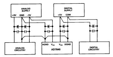
Figure 24. Power Supply Grounding Practice
