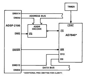
Figure 15. AD7840-ADSP-2100 Parallel Interface
