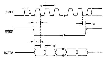
Figure 8. Serial Mode Timing Diagram
