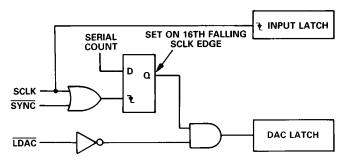
Figure 9. AD7840 Simplified Serial Input Control Logic
